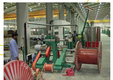
■ Rewinding line from basket Pay-Off to the Take-Up FT-1250. From 400 mm reel up to 1250 mm reel dia.
