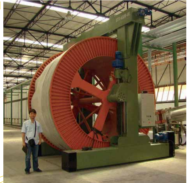
Belt wrap capstan for rubber stripe feeding
