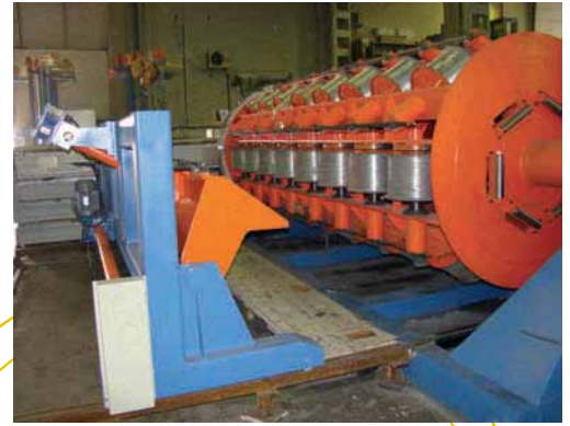
■ Armouring machine ARM-48/400 with automatic side loading unit
