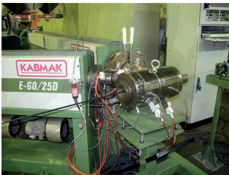
■ Cross Head CH-45/2 with vacuum adapter for natural+skin application
