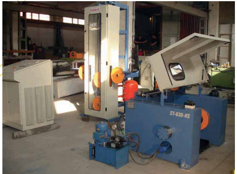
■ Single spooler Take-Up ST-630-HS with dancer unit for rod drawing machine up to 35 m/sec.
