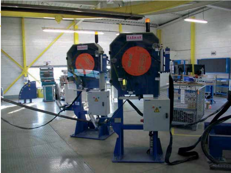
Vertical Caterpillar and cable cutting unit for reel change-over
