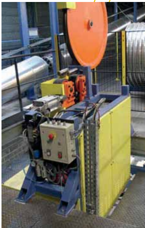
Vertical Caterpillar and cable cutting unit for reel change-over
