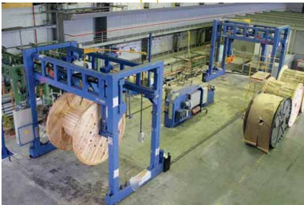
■ Portal Pay-Off PP-4000-D and Take-Up PT-4000 up to 30 tons and 4 m reel
