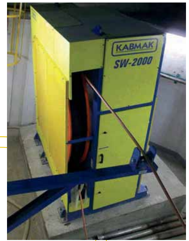
■ Belt Wrap Capstan BWC-2000 for CV line
