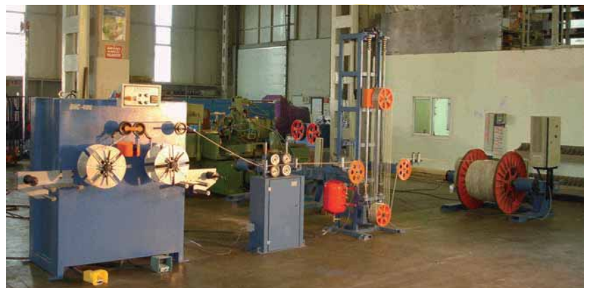
■ Double Head Coiler DHC-400 for multi core cable
