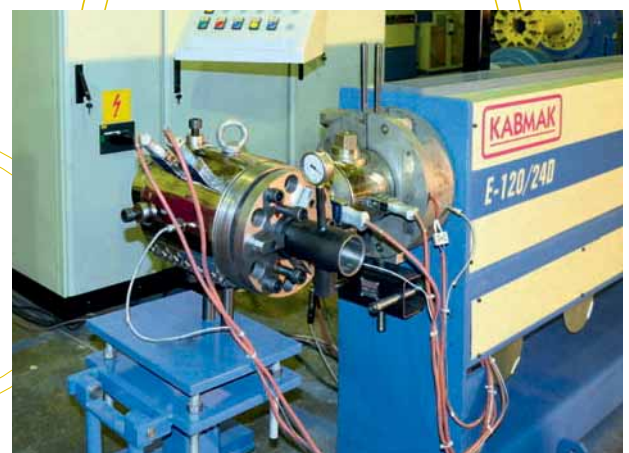
■ Cross Head CH-45/2 with vacuum adapter for natural+skin application
