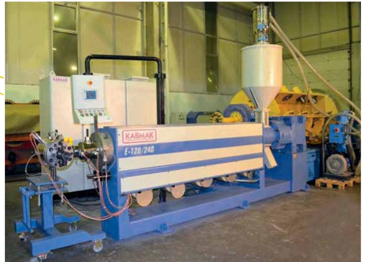
■ Extruder E-120/25D for PVC, XLPE, PE, HFFR
