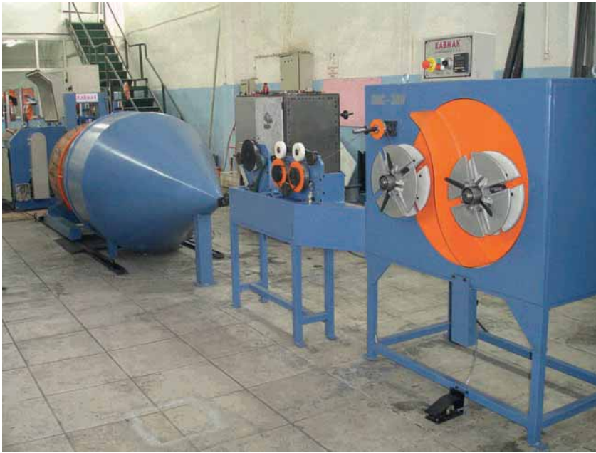
■ Double Head Coiler DHC-300 for single core cable
