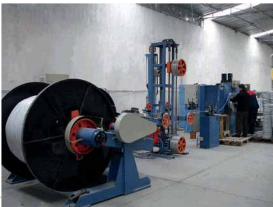
■ Double Head Coiler DHC-600 for multicore cable
