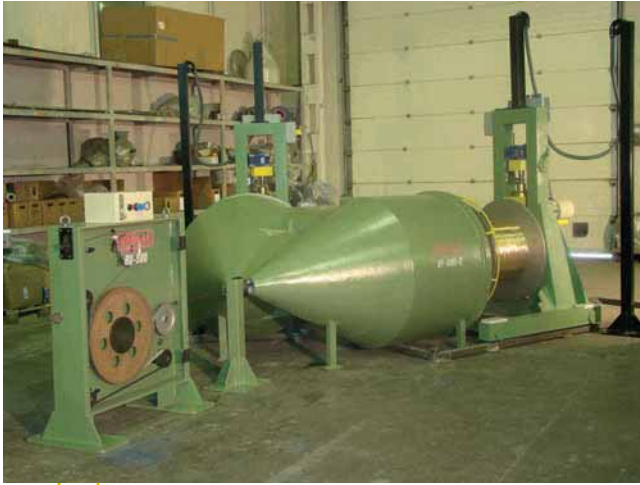
■ Dual Flyer Pay-Off with electromagnetic hysteresis brake
